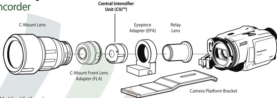
5. Mount the camera to the rear of the Platform Bracket by **loosely** threading the captive thumbscrew into the camera's tripod mount.
