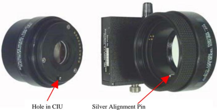
4. Thread the Eyepiece to the back of the 9350EPA about half way.
