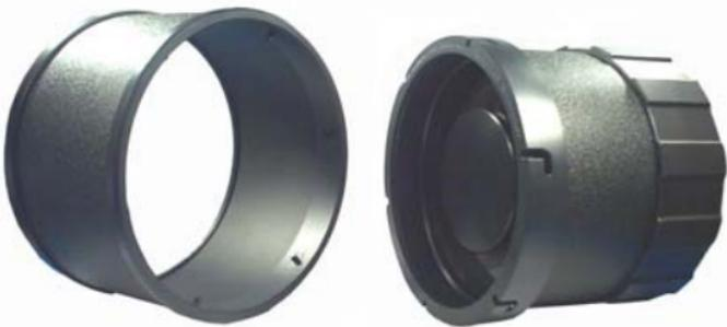
3. Reverse the hood and align the pins with the slots in the lens. Twist clockwise to lock in place.
