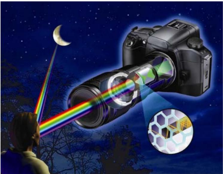
1. The very dim light reflected by scenes at night (lower than 0.1 lux) is focused by an objective lens onto a highly sensitive
