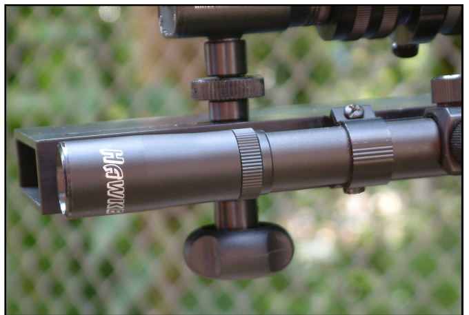
4 x 20 Finder Scope with cross hair mounted on Picatinny rail (rail fitted to both sides of PROMS).
