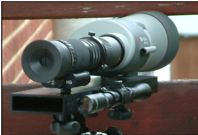
PROMS with optional PNP Night Scope Module for naked eye image intensified operation
