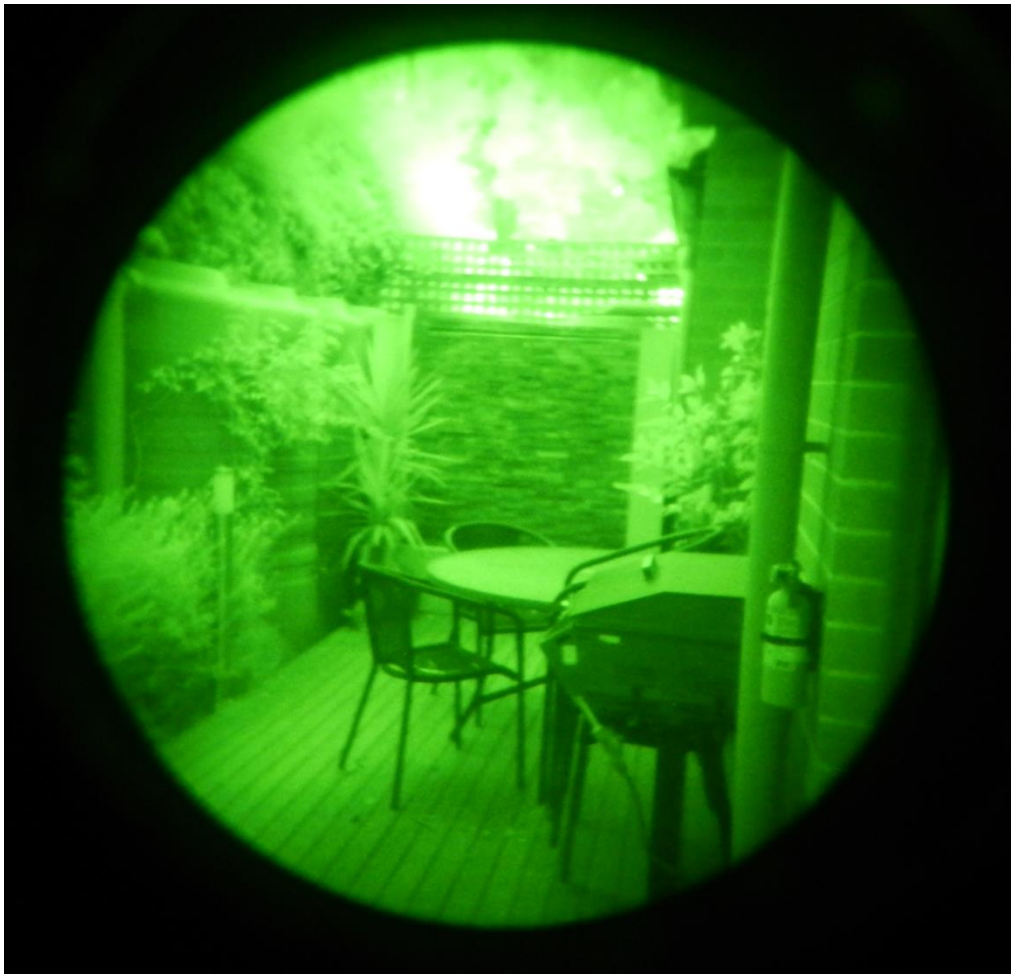
PNP-MC XR5 AUTOGATED – bench test 'Burn-in' negligibly detectable at night
